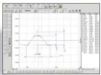
With a software option, TURBO CONTOUR allows you to evaluate leaks on seals.
