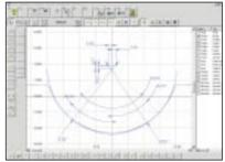
The evaluation function offers you the possibility of carrying out detailed, two-dimensional evaluations of any profile segments of the measured contour.
